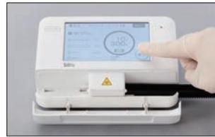
③ Press START, place the test strip and measure.
